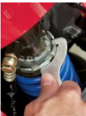
Set your rear sag to 25mm for the track or 30mm for the street.
