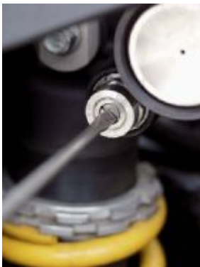
Set your compression damping adjusters to the midpoint of their range
