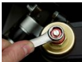
Front sag should be no less than 25mm for the track, 30mm for the street. Some bikes come with extra front sag built in; for now, don't worry if you have too much.
