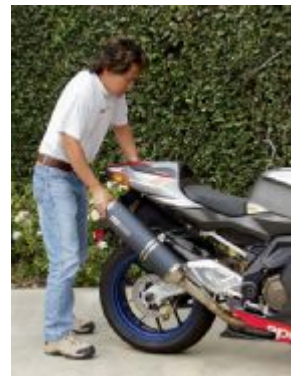
Push down on your tailsection and let the rear end rise. Again, it should take approximately one second for it to return by itself.
