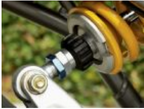
Adjust the rear rebound at the bottom of the shock. This shock also has a ride height adjuster--the large hex nuts--built in.
