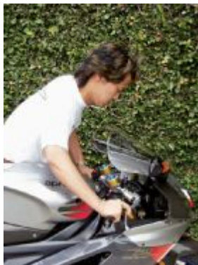
Rebound damping must be set by feel. Push down on the front end and let it rise on its own. It should take approximately one second for it to return to its original position.
