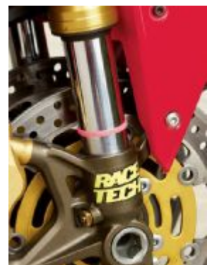
Use a zip-tie on a fork tube to keep track of how close your suspension is to bottoming.
