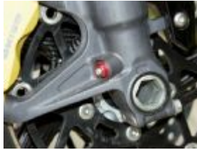
Front compression damping is adjusted at the bottom of the fork.
