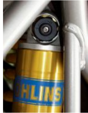
The rear compression damping adjuster is usually at the top of the shock or on the reservoir.
